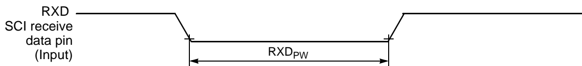
Figure 10-12 RXD Pulse Width
