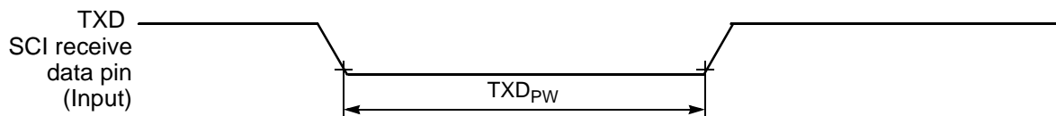
Figure 10-13 TXD Pulse Width
